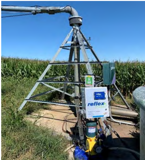
Figure 3. Center-pivot system equipped with a variable rate fertilizer injection pump.
