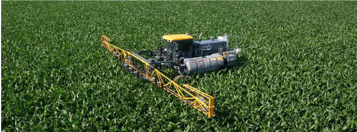
Figure 2. High clearance applicator equipped with OptRx ® crop canopy sensors, GPS, and drop nozzles.
