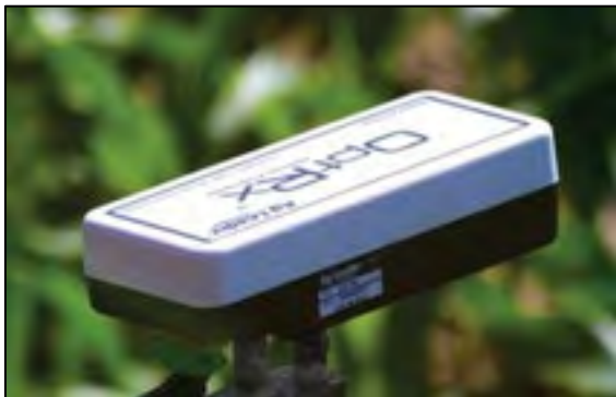
Figure 1. Active crop canopy sensor positioned over corn canopy.
