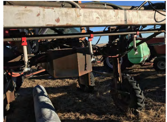
Figure 1. Modified blower used to apply potash.
