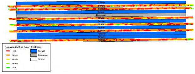
**Figure 2.** Nitrogen rate applied to Project SENSE N Management treatments based on NDRE captured with the crop canopy sensors and displayed in *Figure 1*.
