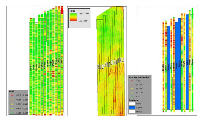
**Figure 1.** NDRE (normalized difference red edge) index obtained using crop canopy sensors mounted on a high clearance applicator for the plot area on July 10, 2017.
