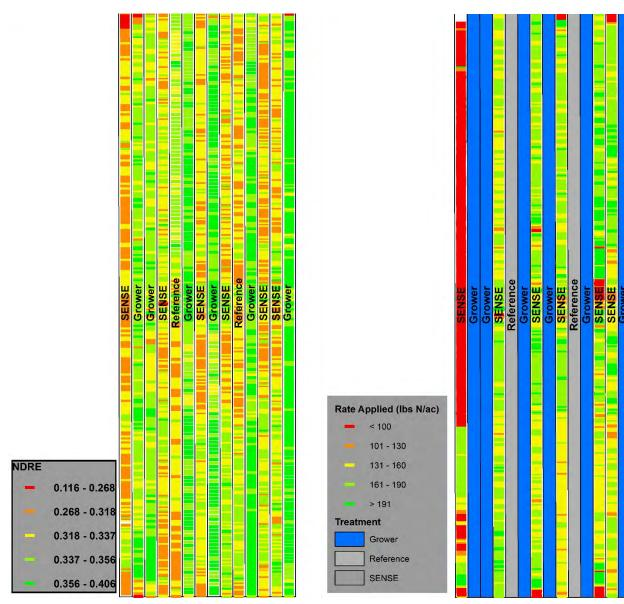
**Figure 1.** NDRE (normalized difference red edge) index obtained using crop canopy sensors mounted on a high clearance applicator for the plot area on June 26, 2017.
